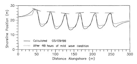
Fig. 6. Test for decay of tombolos.
