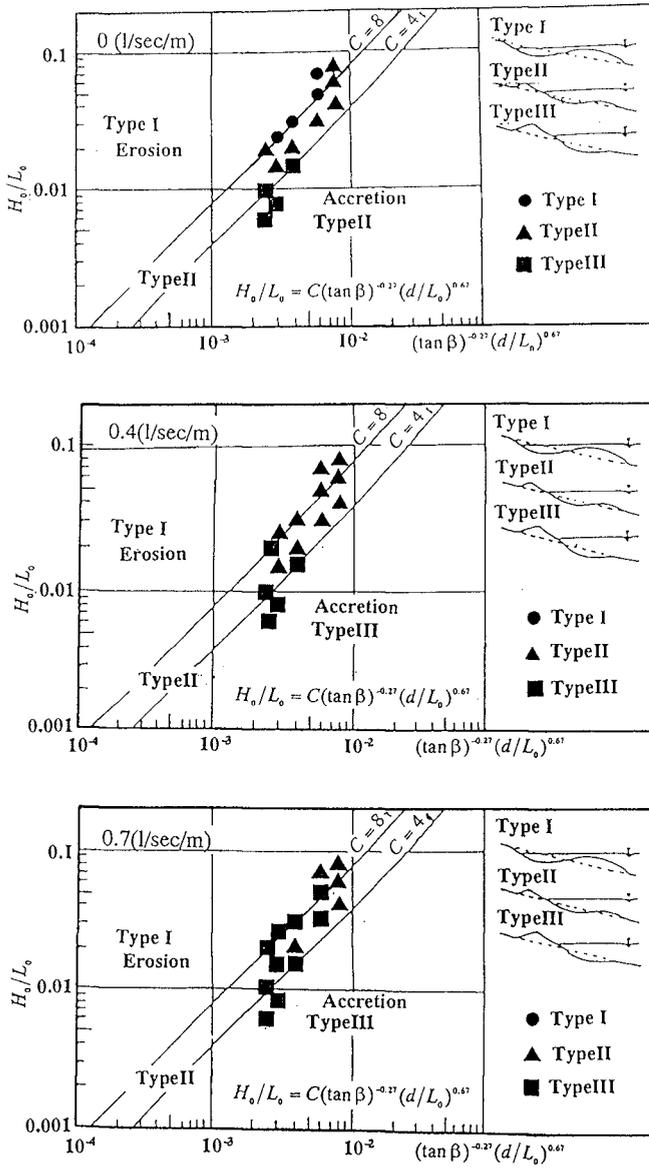
Figure 14 Change of beach type with discharge
