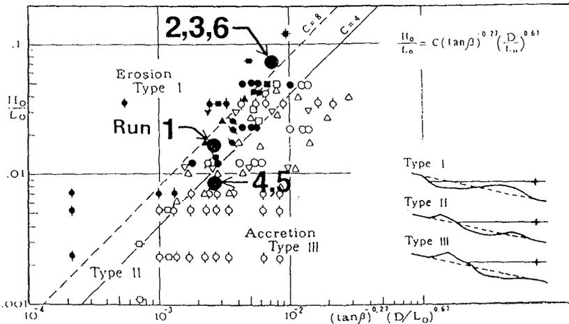
Figure 4. Classified laboratory beach profiles(Sunamura and Horikawa, 1974)
