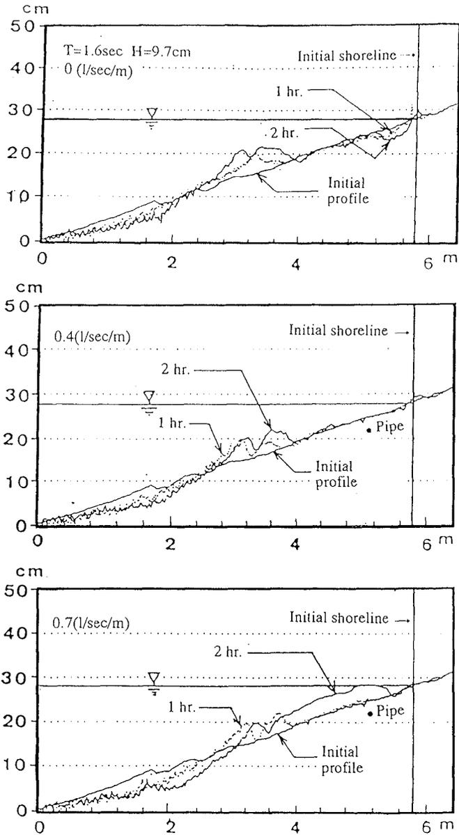
Figure 13 Changes of beach profile with discharge
