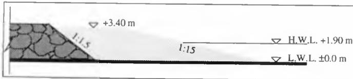
*Fig. 3.* Typical design cross section of the beach
