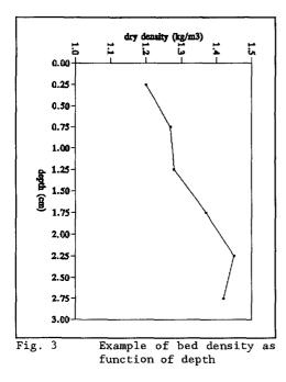
The samples are weighted in order to obtain the wet bulk density, dry bulk density, moisture content and voids ratio.
