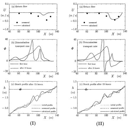
Figure 5: Simulation results for Case 3-3 with the undertow model of (I) Sato et al. and (II) Okayasu et al..
