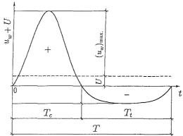
Figure 3: Definitions for the near-bottom velocity profile.
