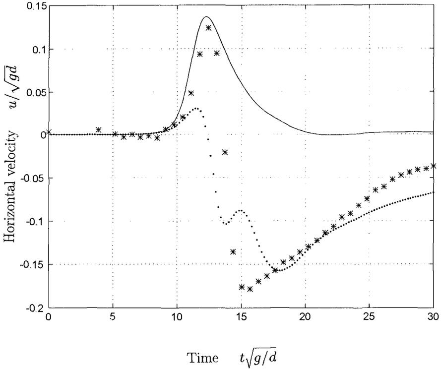
Figure 6: Comparison of horizontal water particle velocities at location P near the surface of the shoreward breakwater. The breakwater height to water depth ratio is 0.5 and the solitary wave height to water depth ratio is 0.3.
