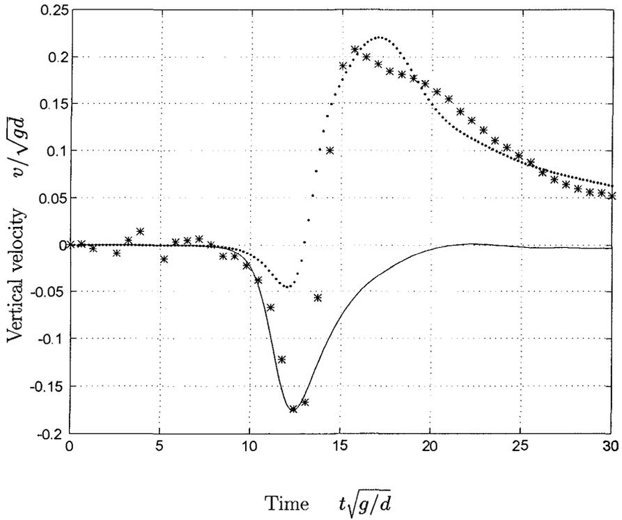
Figure 7: Comparison of vertical water particle velocities at location P near the surface of the shoreward breakwater. The breakwater height to water depth ratio is 0.5 and the solitary wave height to water depth ratio is 0.3.
