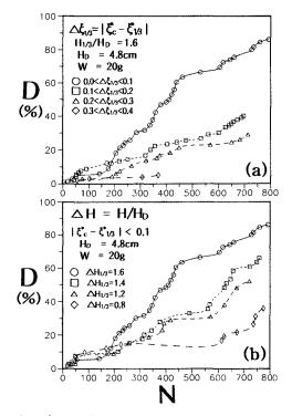
Fig. 4. Storm duration effects on the failure of rubble mound structures with the resonance indexes  $\Delta \xi^*_{1/3}$  (a) and  $\Delta H_{1/3}$  (b).
