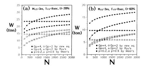
Fig. 8. An example of design weight of rubble unit in relation to storm duration.
