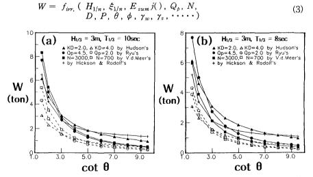
Fig. 1. Design weights of rubble units in relation to the slope angle by various formulas.
