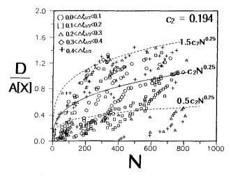
Fig. 6. Variation of damage level according to the storm duration.
