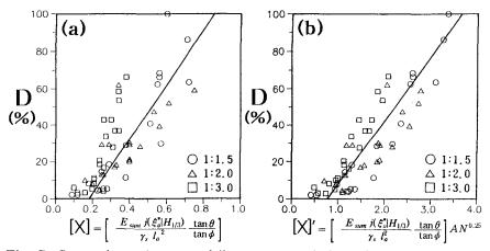
Fig. 7. Comparisons between failure characteristics with respect to the previous irregular force parameter (a) and the modified parameter (b).
