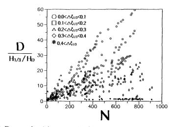
Fig. 5. Damage level increase of rubble mound structures according to the resonance indexes and the storm duration effects.
