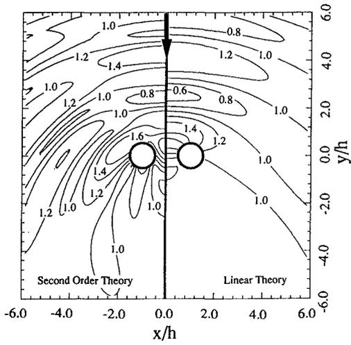
Fig.6 Maximum wave amplitude distribution near double circular cylinders.
