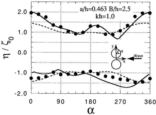
Fig.5 Wave runup and rundown around double circular cylinder.
