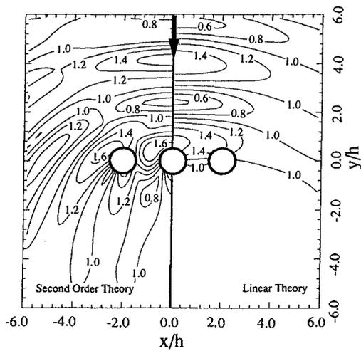
Fig.7 Maximum wave amplitude distribution near triple circular cylinders.
