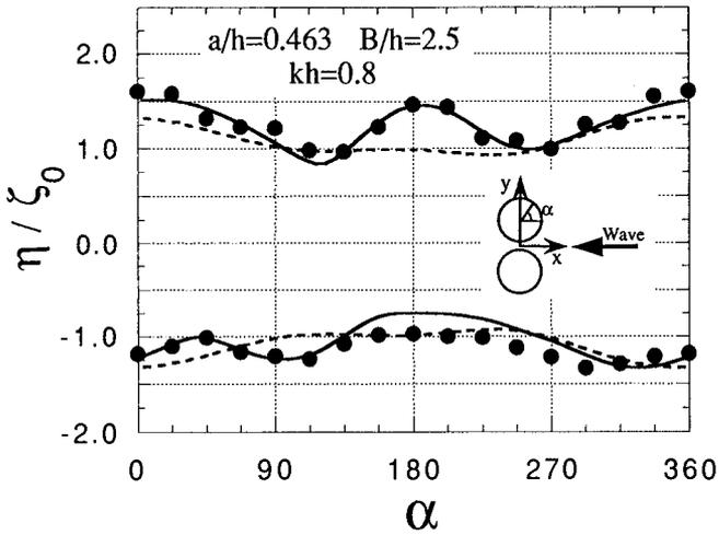
Fig.4 Wave runup and rundown around double circular cylinder.
