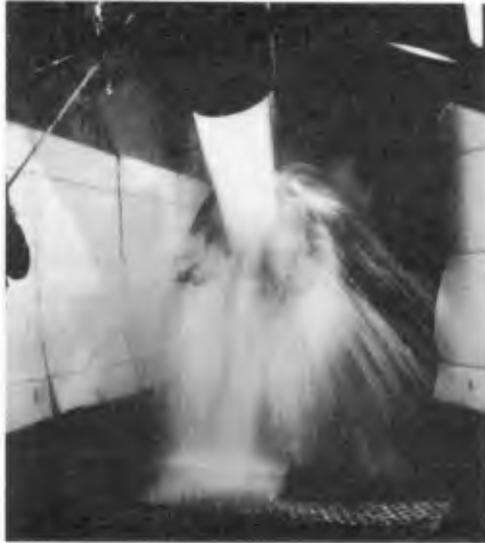
**Photo 1** Assessing first author's stability under water jets; a ballasted manikin (on the left) is waiting for its turn.
