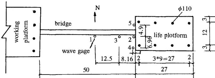
Fig.1 The arrangement of the wave gage array
