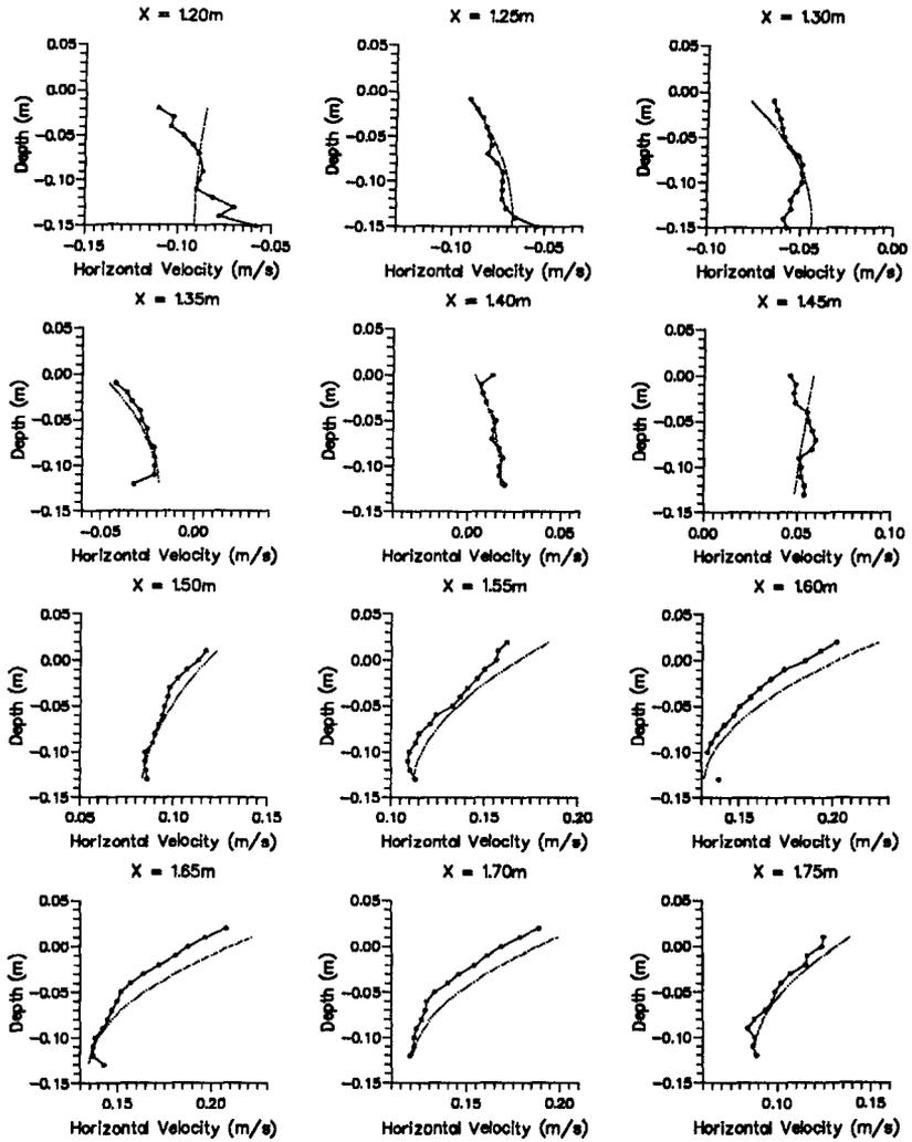
Figure 8: Calculated and Measured Velocity Profiles at Different Horizontal Positions ( $x$ ) in the 1s wave on a 1:30 Beach.
