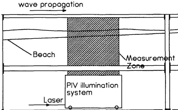
Figure 1: The Flume and PIV Illumination Section.
