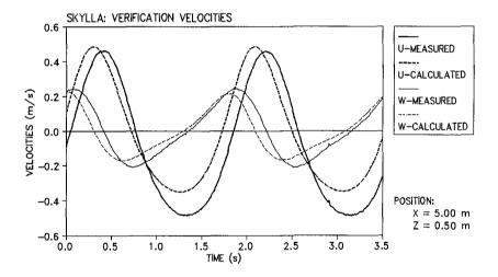
Figure 15 Comparison of measured and calculated velocities; u denotes horizontal velocities, w denotes vertical velocities
