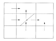
Figure 6 Virtual velocity components for a cell of category 4
