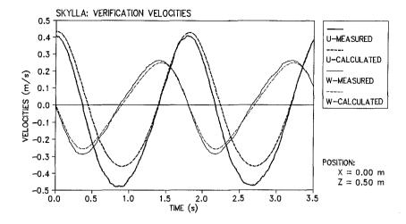
Figure 14 Comparison of measured and calculated velocities; u denotes horizontal velocities, w denotes vertical velocities
