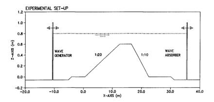
Figure 9 Bottom topography used in wave flume
