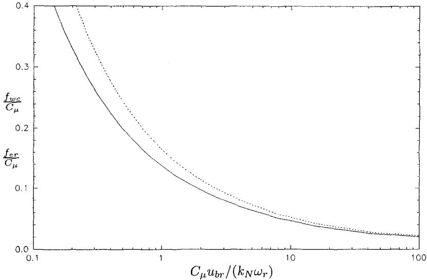
Figure 1: Generalized Friction Factor Diagram for Waves in the Presence of a Current. Wave Friction Factor,  $f_{wc}$ , (dashed line), Wave Energy Dissipation Factor,  $f_{er}$  (full line), for the Representative Periodic Wave.
