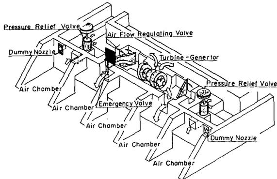
Figure 5 Conceptual View of the Machine Room
