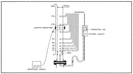
Fig.1: Settling column: experimental set-up.
