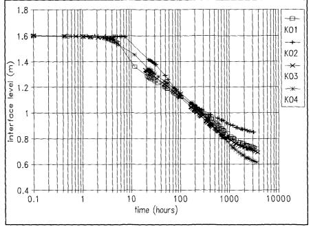
Fig.2: Settling curves for experiments KO1-KO4.
