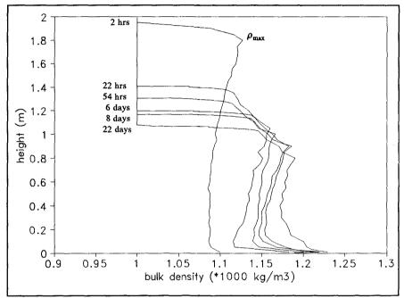
Fig.10: Density profiles for column KO8.
