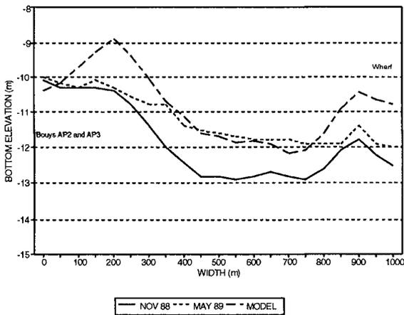
Figure 9.- Bottom elevation results along a cross section of the maneuvering zone. Comparison of computed elevations with measured data.
