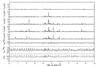
Figure 3- A 10-minute time series for the middle-surf-zone location (6). From the bottom, the hydrostatic approximation to sea level (h), cross-shore (U) and longshore (V) water velocities at 50 cm above the bed, and sediment concentrations (ppt) at 13, 19, 31, and 61 cm above the bed. The time period corresponds to 2 through 12 minutes shown in Figure 2.
