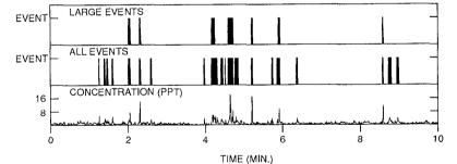
Figure 6- Application of suspension event definitions to the 10-minute series in Figure 3. From bottom to top are: 1) the concentration time series, 2) all events shaded, 3) large events shaded.
