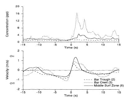
Figure 11- Ensemble averaged velocity and concentration for all events at measurement locations in the bar trough, bar crest, and middle surf zone. The time series are averages of velocities and concentrations for large suspension events with the velocity zero-upcrossing as the common time reference.
