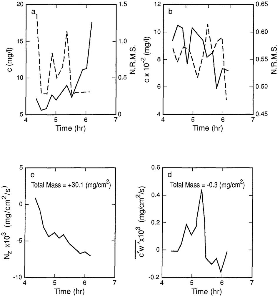
Figure 3. a.) Time Trace of Concentration at 50cm Above Bottom (AB); b.) Time Trace of Concentration at 5cm AB; c.) Time Trace of Vertical Flux,  $N_z$ , at 50cm AB; and d.) Time Trace of Turbulent Flux,  $\overline{c'w'}$ , at 50cm AB.
