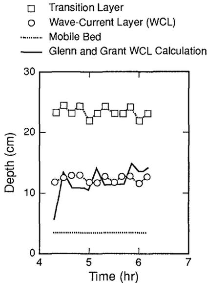
Figure 7. Time Trace of the Heights of the Measured Transition Layer ( $\square$ ), the Measured Wave-Current Boundary Layer ( $\circ$ ), the Measured Mobile Layer ( $\cdots$ ) and the Calculated Wave-Current Layer ( $\text{—}$ ).
