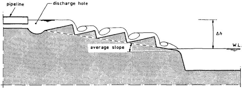
Fig.7. Terrace formation on fill above water level.
