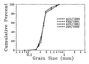
Fig. 4.- "Master sample" grain size distribution.
