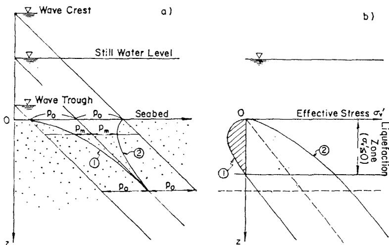
**Fig.1 Momentary liquefaction of seabed due to waves
