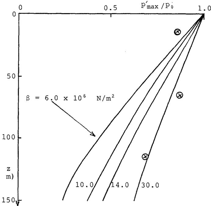
**Fig.5 Comparison of calculated porewater pressure(—) with measured porewater pressure(x)**
