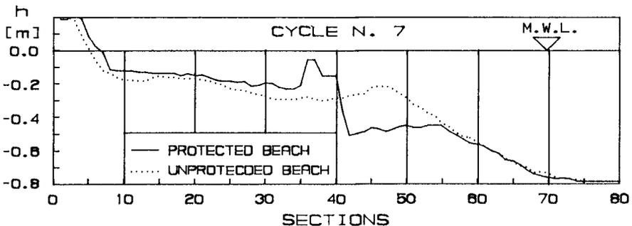
Figure 8. Comparison between protected and unprotected beach profiles.
