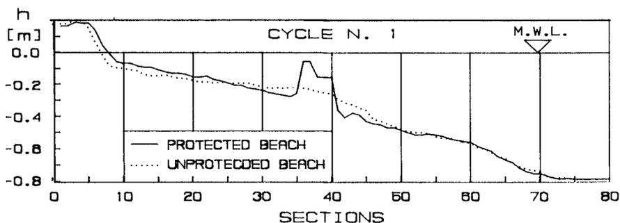
Figure 6. Comparison between protected and unprotected beach profiles.
