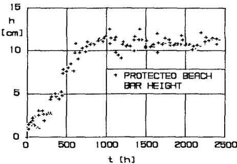
Figure 18. Evolution of bar depth in protected beach.
