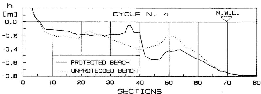
Figure 7. Comparison between protected and unprotected beach profiles.
