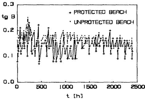
Figure 11. Evolution of swash-zones slope.
