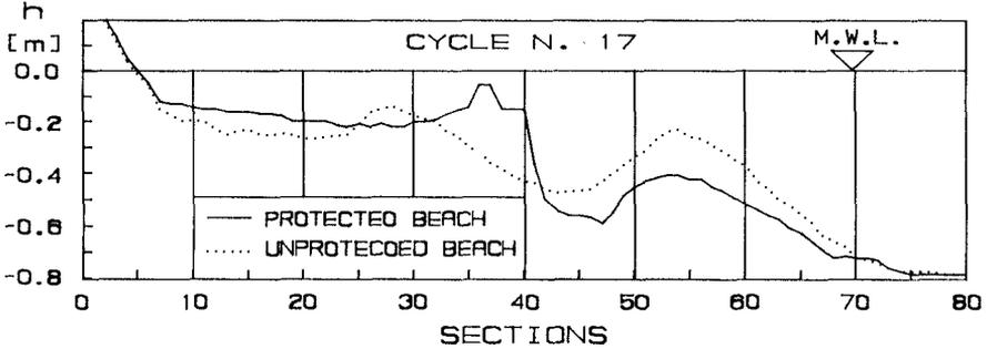
Figure 9. Comparison between protected and unprotected beach profiles.
