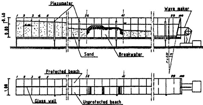
Figure 1. Experimental channel.
