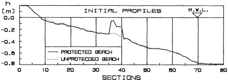
Figure 3. Comparison between protected and unprotected beach profiles.
