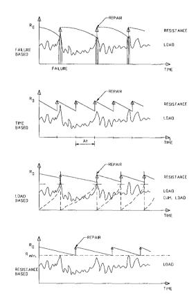
Fig. 1 Corrective maintenance and preventive maintenance governed by various triggers
