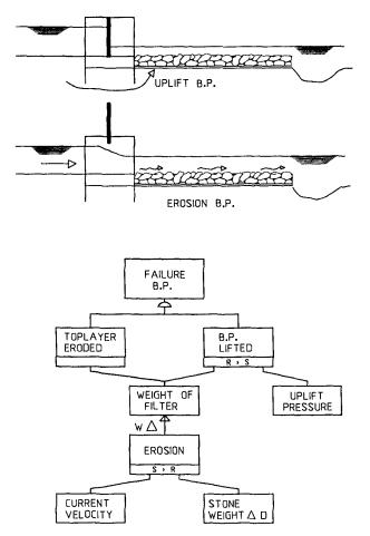
Fig. 8 The two failure modes of the bottom protection The transport relation has the following form T = 1260  $(U - 2)^2$  kg/m2 per year for U>2 m/s and T=0 elsewhere.
