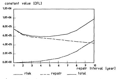
Fig. 11 Total expected cost as a function of the repair interval
