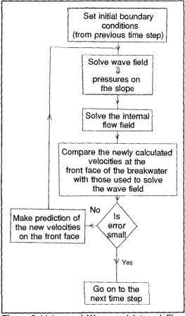
Figure 3 Linkage of Wave and Internal Flow Models.
