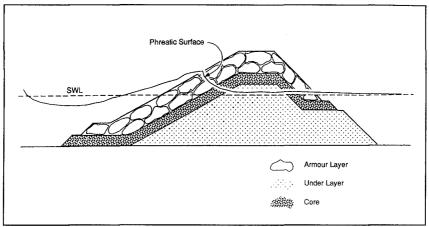
Figure 1 Wave action on a rubble mound breakwater.
