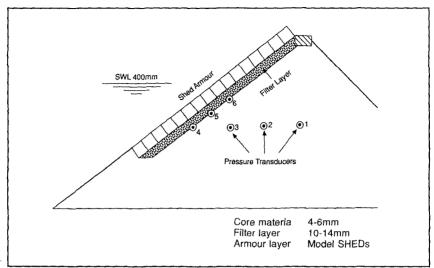
Figure 4 Locations of the pressure transducers.
