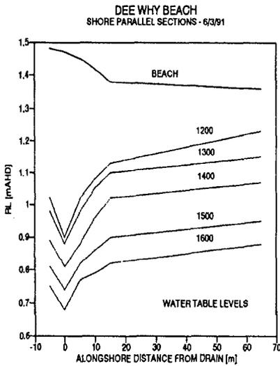
**Figure 5** — Effects of a single drain on the watertable at various times (EST)
