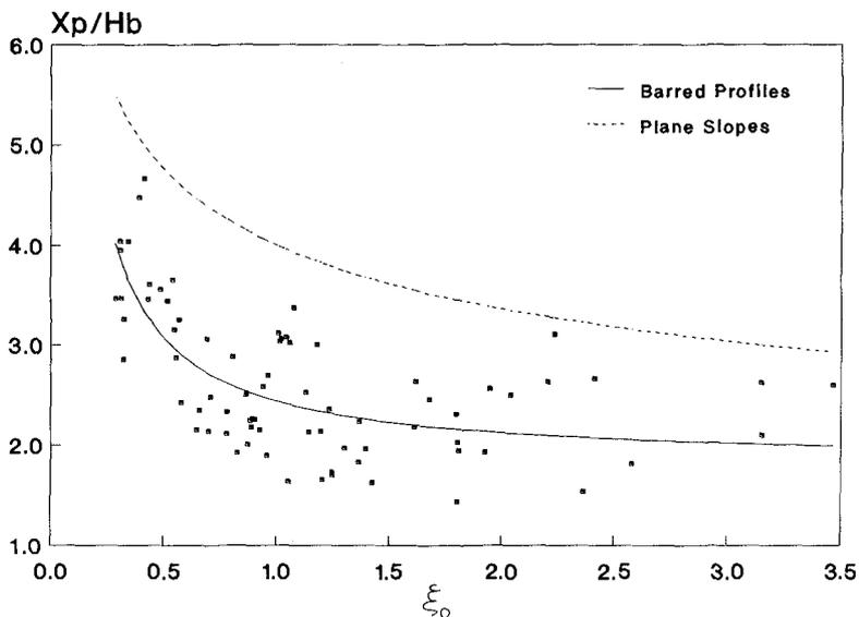
Fig. 2. Plunge distance on plane and barred slopes (Smith & Kraus 1991)
