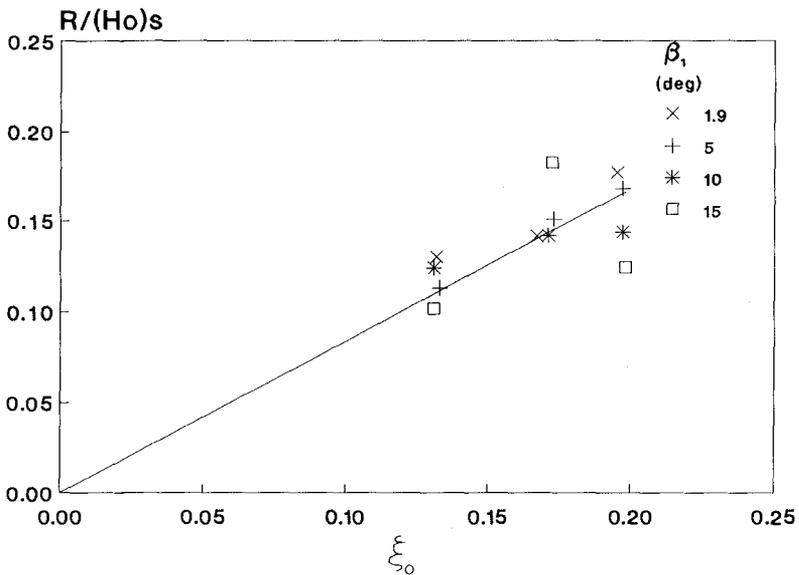
Fig. 7. Runup on barred and plane slopes (random waves)
