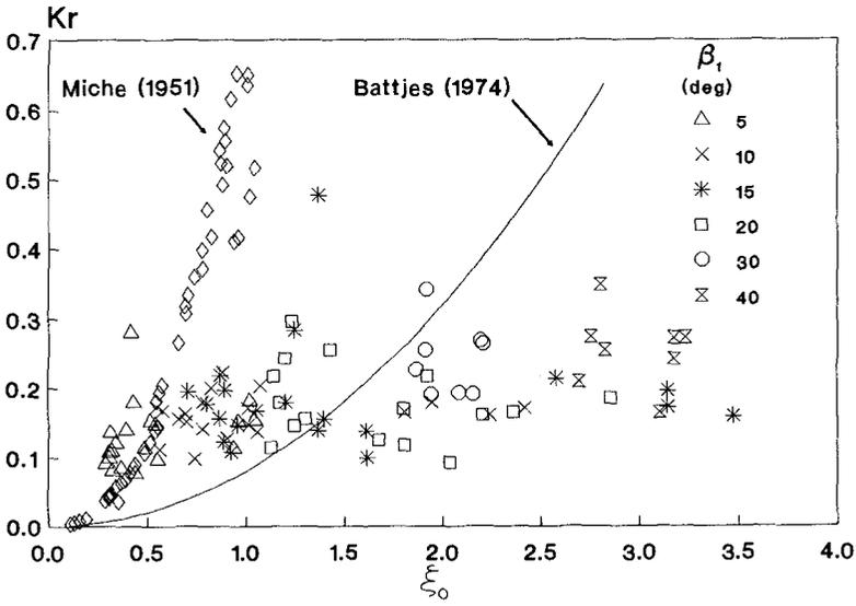
Fig. 4. Measured reflection coefficient vs. surf-similarity parameter
