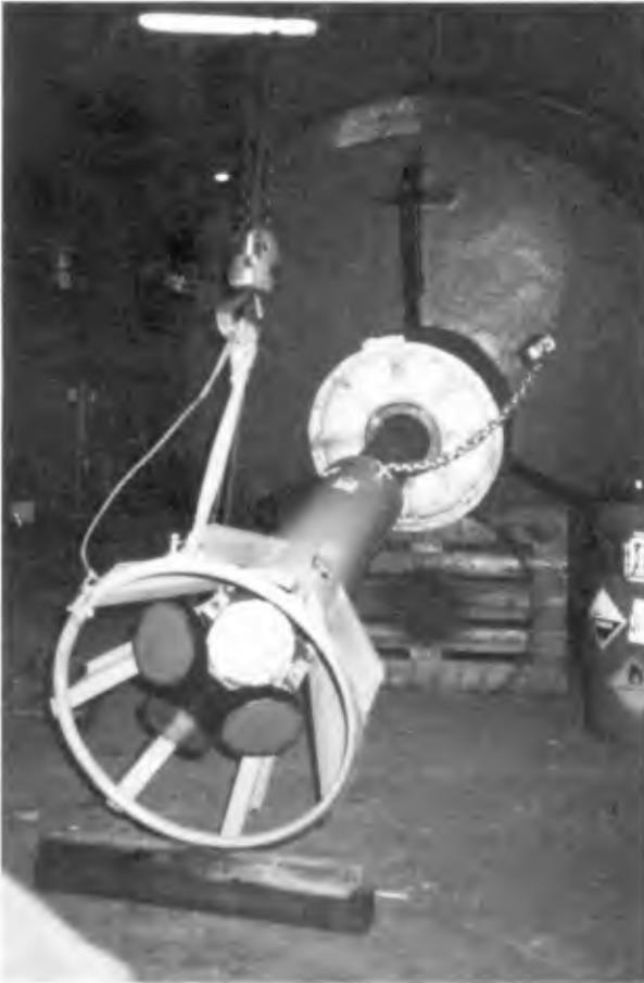
Fig. 7. An ADCP current meter installed below the WAVESCAN buoy.
