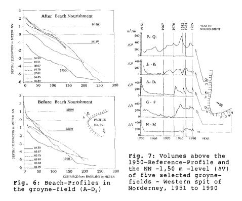
structures against failure during storm floods. To meet this target the volume calculation can be restricted to the beach part above NN -1,50 m - level, that's about MLW. This practical engineering approach is appropriate. There will be no discussion on the complicated cross- and longshore processes within enlarged boundaries.
