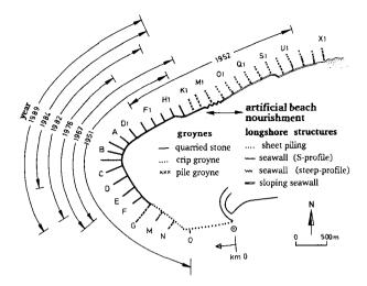
Fig. 3: Combined Protection System on Norderney-island
