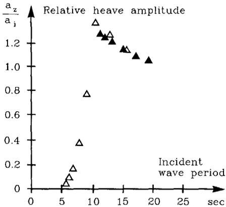
Figure 7. Comparison of calculated and experimental heave motions of the barge in beam waves.  $a_z$  and  $a_i$  are the amplitude of heave and the incident wave, respectively.
