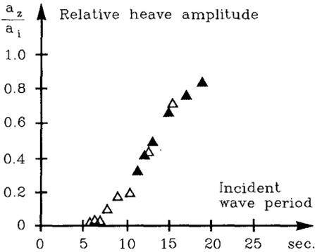
Figure 10. Comparison of calculated and experimental heave motions of the barge in head waves.  $a_z$  and  $a_i$  are the amplitude of heave and the incident wave, respectively.
