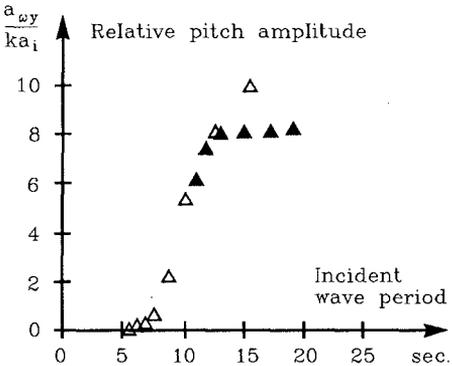
Figure 11. Comparison of calculated and experimental pitch motions of the barge in head waves.  $a_{wy}$  and  $a_i$  are the amplitude of pitch and the incident wave, respectively,  $k$  is the wave number  $k = 2\pi/L$ .
