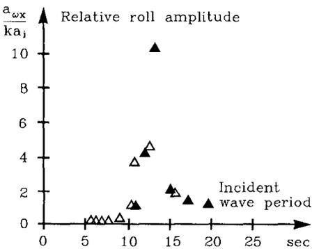
Figure 8. Comparison of calculations and experimental roll motions of the barge in beam waves.  $a_{wx}$  and  $a_i$  are the amplitude of roll and the incident wave, respectively,  $k$  is the wave number  $k = 2\pi/L$ .
