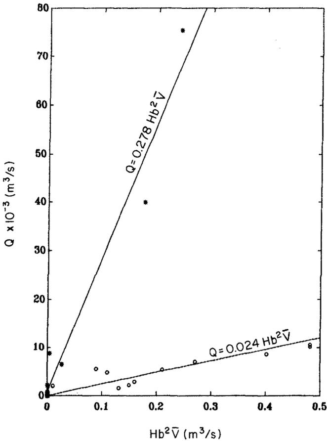
Figure 4. Volumetric transport rate.
