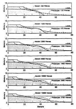
Figure 3: Comparisons between GWK and  $\frac{1}{10}$  Scale Model with  $N_{\delta} = N_{\lambda} = 10$  and  $N_{t} = 1$  (from Dette and Uliczka, 1986).
