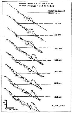
Figure 1: Comparison between Saville and Kriebel (from Kriebel, et.al. 1986).
