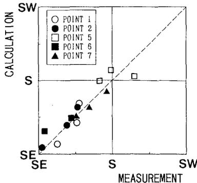
Fig.5 Comparison between the measured and the calculated principal wave direction
