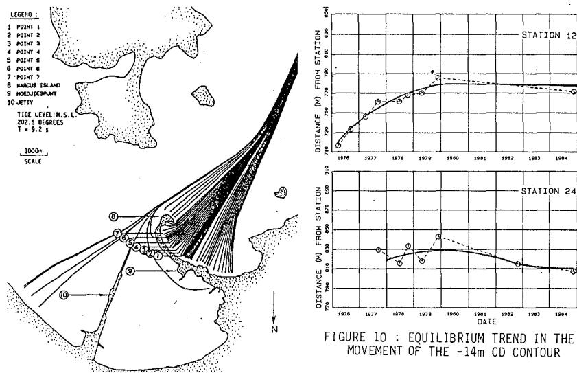
FIGURE 10 : EQUILIBRIUM TREND IN THE MOVEMENT OF THE -14m CD CONTOUR
