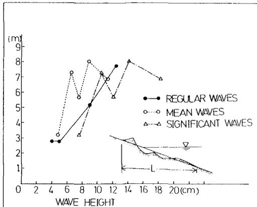
Fig.14 The length of on-offshore depth change limits.
