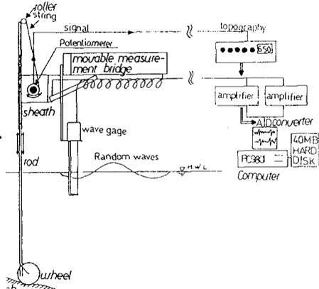
Fig.3 Automatic measurement system for wave and topography.
