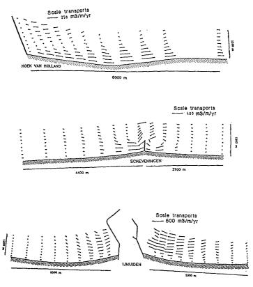
Figure 4.Resulting tidal sediment transports near the harbors.
