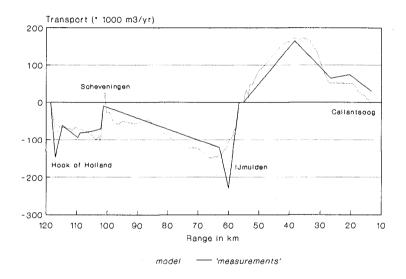
Figure 6. Calibration of the longshore transports.
