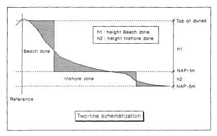
Figure 2. Two-line schematization
