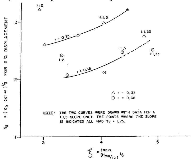
**Figure 5.** Effect of Armour Slope on Stability
