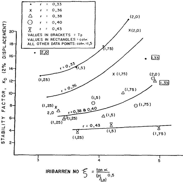
Figure 6. Design Curve for 2 per cent Displacement
