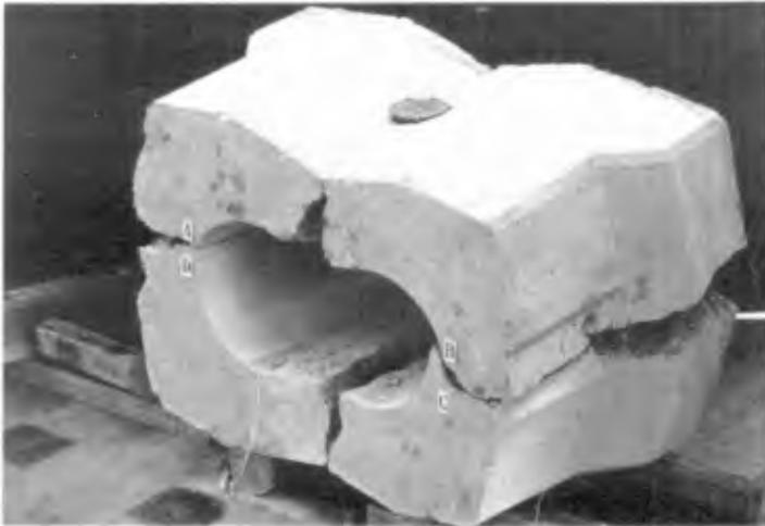
Figure 3. Block after the static loading test
