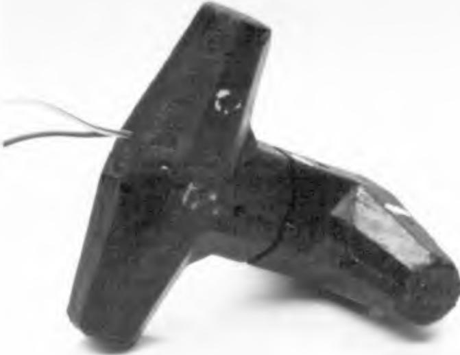
Figure 1. The Dolos Armor Unit Load Cell
