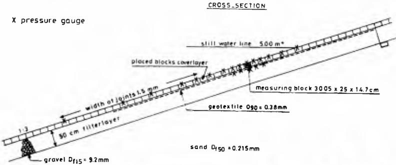
Figure 1. Cross section of revetment II West
