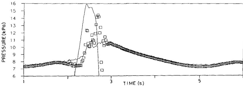
Figure 10. Measured uplift pressure compared with block movement
