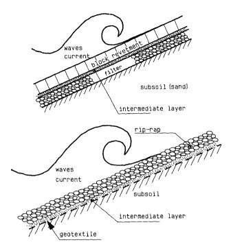
Fig 1. Wave attack on revetments
