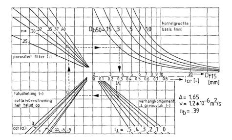
Figure 9 Design diagram for granular filter interface
