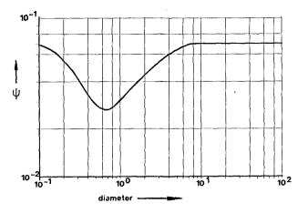
Figure 4 Shields parameter.
