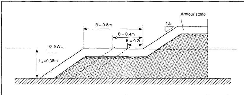
Figure 2 Bermed slopes tested
