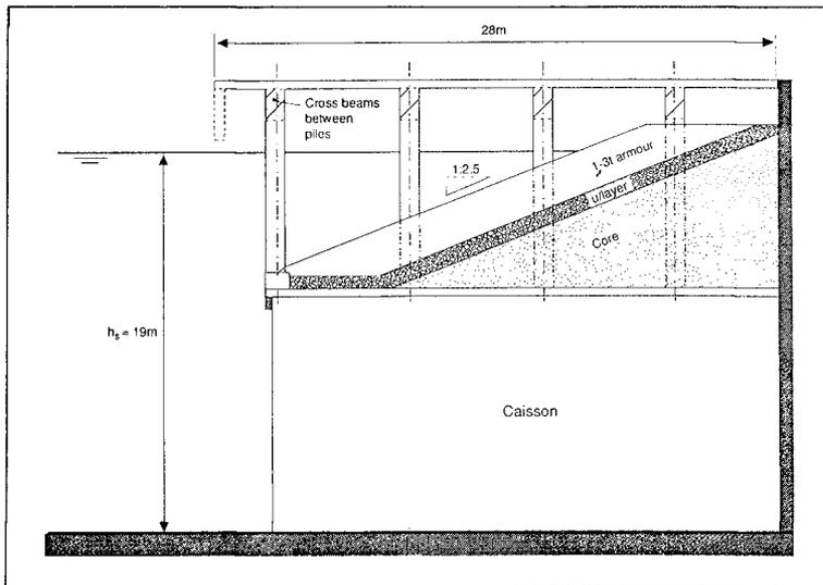
Figure 9 Coal berth quay, option A1/A2
