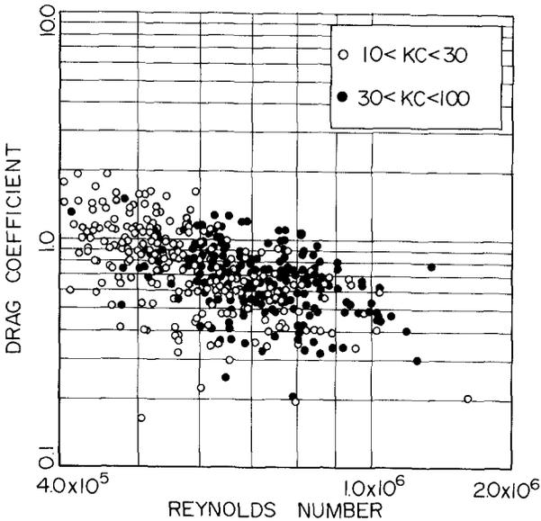
Fig.6 Relation between drag coefficient and Reynolds number
