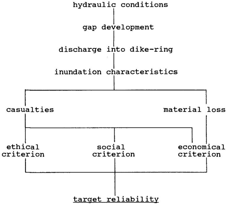
Figure 3: Determination of target reliability
