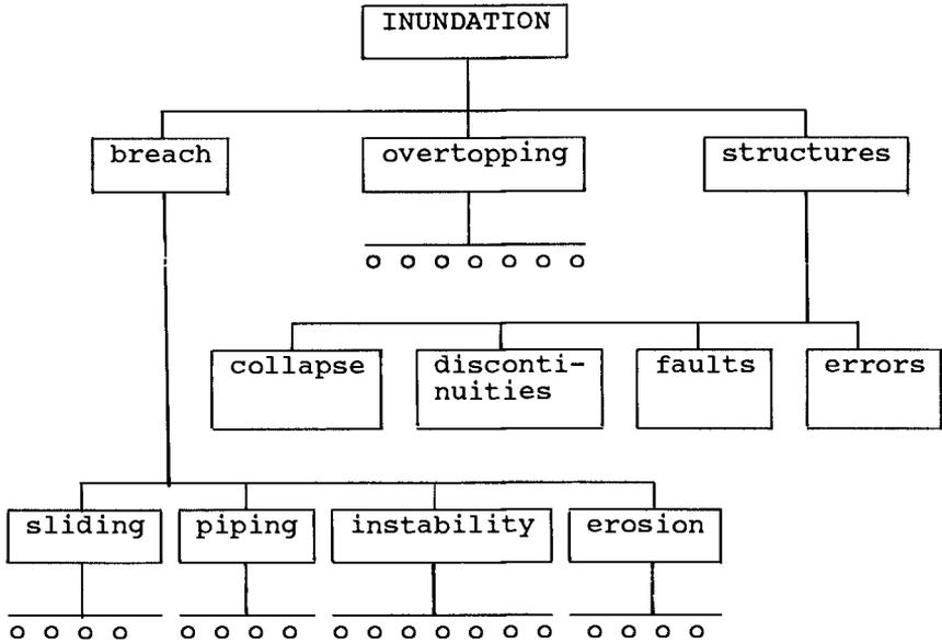
Figure 8: Failure Tree for a Dike-ring
