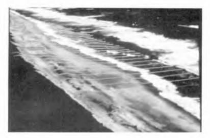
Figure 1. Example video frame showing waves in the nearshore and run-up. Lines across the beach represent surveyed beach profiles. For automatic digitization, the computer searches out along each line (starting with the left hand tick) until it finds the run-up (marked by the right-hand tick). 39 transects are shown.
