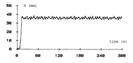
Fig.5 Time series of wave heights 5m from the paddle when waves are added to a steady current.
