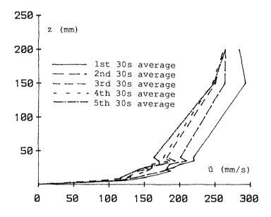
Fig.1 Boundary layer profiles of horizontal velocity at 30s intervals after the superposition of waves [T=ls;].
