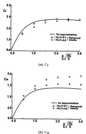
Fig. 9 Variations of  $C_F$  and  $C_M$  with  $(a/h)\sqrt{H_0/h}$ .
