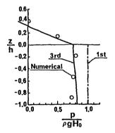
(b) Distribution of hydrodynamic pressure under the wave crest Fig. 4 Comparisons with the corresponding approximation for  $H_0/h = 0.4$ ; O, numerical result; — , third approximation; ---, first approximation.
