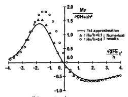
(b) overturning moment Fig. 7 Temporal variations of horizontal force and overturning moment for  $(a/h)\sqrt{H_0/h} = 2.0$ .
