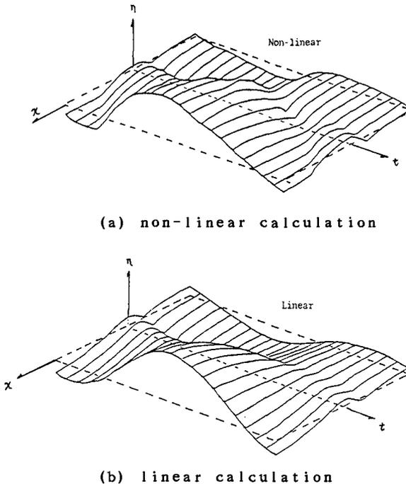
Fig. -3 Numerical simulation of Bore-like surf beat
