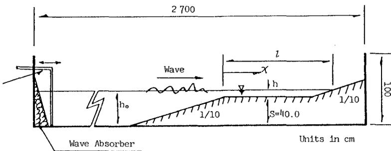
Fig.-4 Experimental equipment
