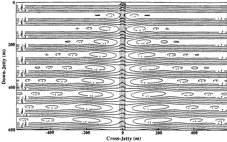
Figure 2: Normalized, instantaneous surface elevation field. Incoming wave: incidence angle =  $0^\circ$ , period = 14 sec, height = 0.8 m, length = 120 m. Model jetty: core width = 32 m, stone diam. = 1.25 m, porosity = 0.45. The origin of the semi-infinite jetty is at (0,0).
