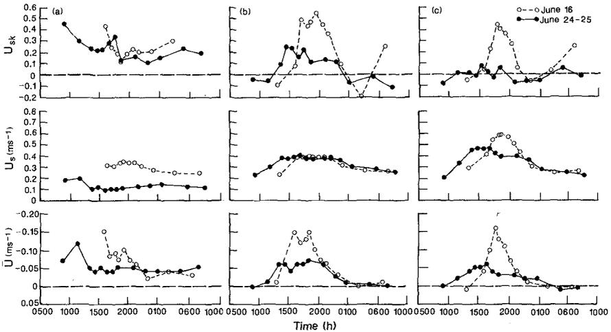
Figure 4. Temporal variation of near-bed (0.10 m) velocity parameters,  $\bar{u}$ ,  $u_s$ , and  $u_{sk}$ , during the two storm events: 10 m offshore (a), 65 m offshore (b), and 110 m offshore (c). Note: positive values indicate onshore direction.
