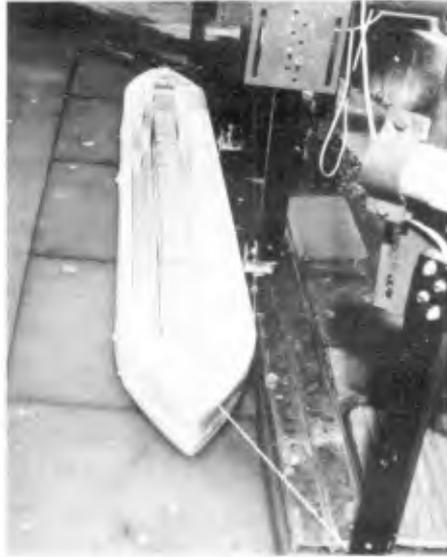
Figure 1. Ship's model moored in harbor's hydraulic model.
